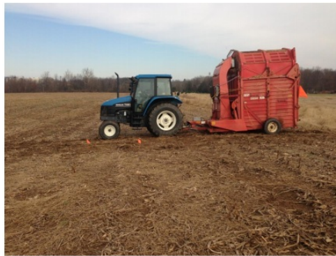
Stover removed with Hess hay stacker.
